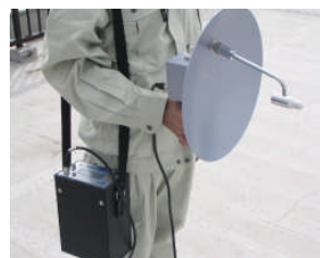
Corona discharge detector in air
