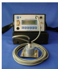
Corona discharge detector in oil
